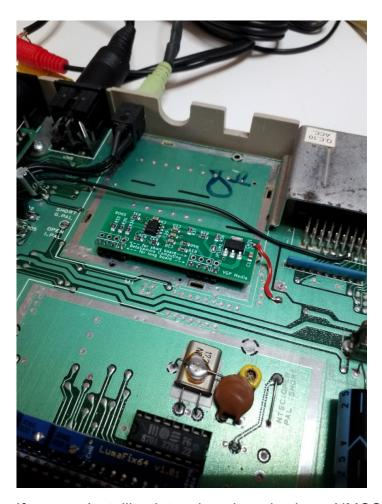
If you are Installing into a long board using a NMOS VIC-II chip then you MUST close **JPLUM1** on the board too, using some solder to join the pads.
