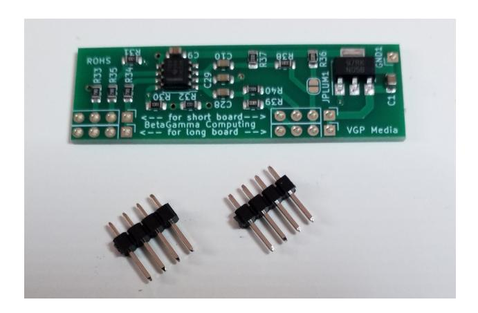
This installation guide describes the installation of the open source C0pperdragon RF modulator replacement and amplifier board for the Commodore 64 microcomputer system.
